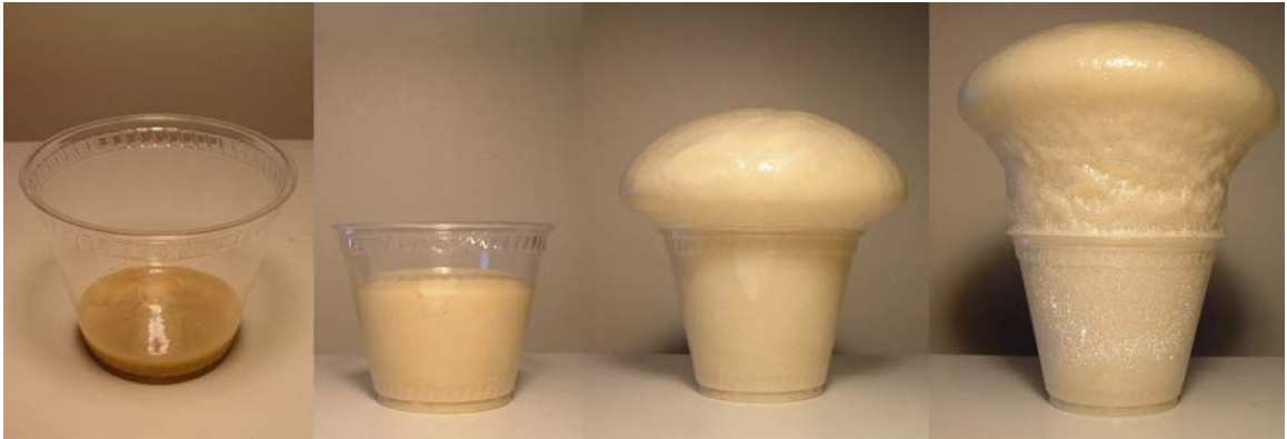
Figure 9.2 Expansion of 2-part polyurethane foam.
