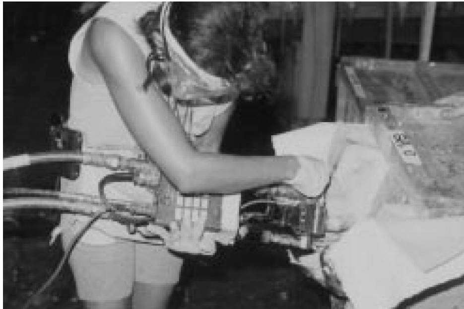
Figure 3.6 Injection of polyurethane foam into mold cavity. [Greene Associates]
