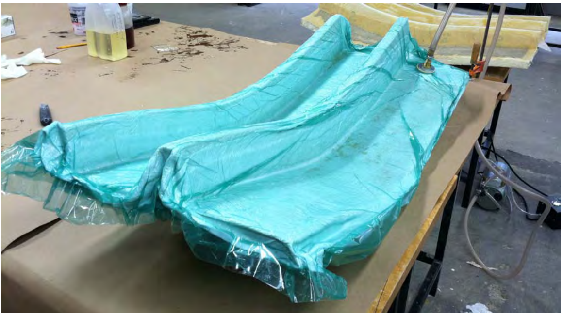
Figure 9.27 Vacuum bag consolidation of rear lamination.
