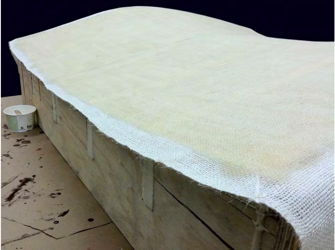
Figure 9.25 Lamination of foam surface.
