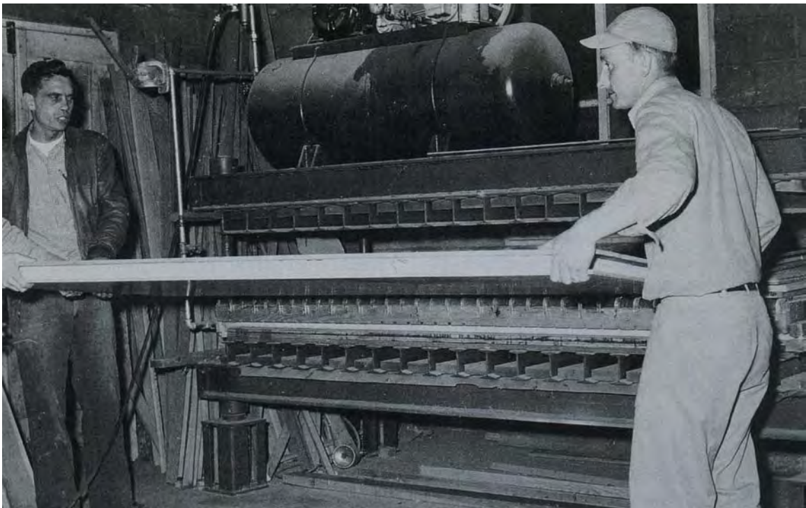
Figure 2.3 Dow Structural Insulated Panel manufacture, 1959. [Morley]
