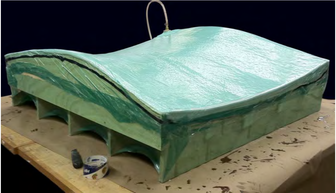
Figure 9.26 Vacuum bag consolidation of front lamination.
