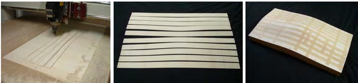
Figure 9.9 3-axis CNC cutting of developable surface strips.
